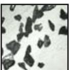
Silicon carbide is the most aggressive media used for micro-abrasive blasting. It has a hardness over 9 on the Mohs' scale, just under diamond. This media is typically used only where very fast material removal is a requirement. Silicon carbide is an excellent abrasive for deburring stainless steel and titanium parts.
