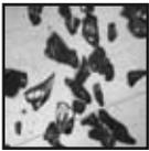
Aluminum oxide is the most commonly used cutting abrasive. The shape and hardness of the particle make it an excellent choice when working with metals or hard, brittle parts. Common uses for aluminum oxide include cutting, deburring and the preparation of surfaces. It is available in a wide range of sizes from 10 to 150 microns.
