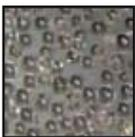
Glass bead is commonly used where the preservation of tight tolerances is critical combined with the need to relieve stresses. It is also used to perform light deburring or to apply a satin-like finish on a part. The spherical shape of the glass bead keeps it from cutting into the surface of the part, so it is commonly used to relieve stresses by "pounding" the part's surface.
